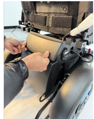
INSTALL THE BATTERY BOX COVER (TOP)
