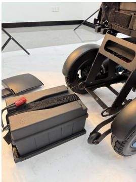
PLACE THE BATTERY IN TO THE TRAY
